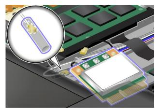
9. Pivot the card until you can snap it into place by pressing the upper side of the connectors, and secure the card with the screw.
